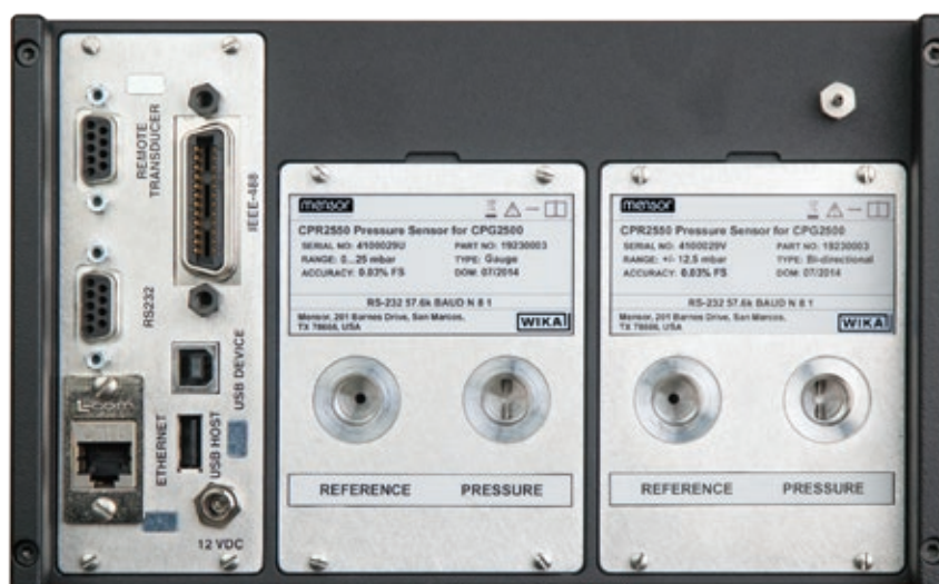
Figure 5.4 A - Two removable gauge transducers installed
